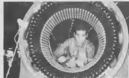
On a training assignment under the Lago Cooperative Education Program, Hubert T. Lopez, an HTS electrical engineering student at Breda, Holland, assists in rewinding an electric motor.
